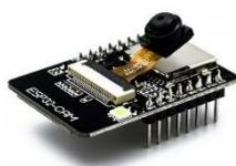
Gambar 2.3. Modul ESP32-CAM
